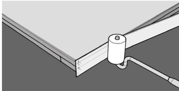
Using a laminate trimmer or router with a laminate bit, trim the excess laminate flush with the edges of your substrate. Where laminate corners meet, use a file to lightly file the corner at a 45° angle to finish.
